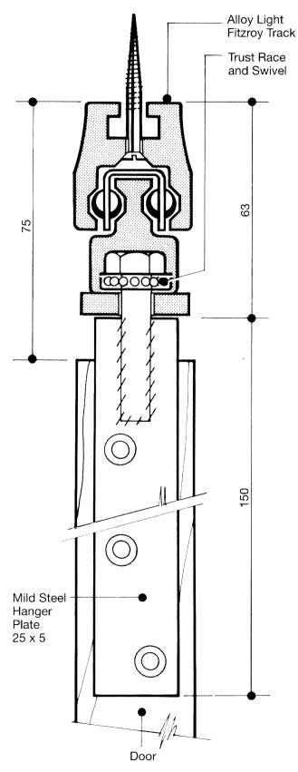
Set out on the sheet is a Bi-fold Door System using the Alloy Light Fitzroy Door Track.
